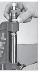
(8) SCREW the bullet seating die in until you feel it touch the case mouth. If no crimp is desired, back
