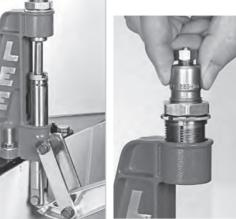
To remove quick-change bushing, rotate the die 1/6 of a turn counterclockwise. lift out. You can add bushing to your next die, or install an additional bushing on the rest of your dies for quick-change convenience.
