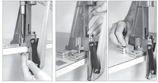
**ATTACH** your press with (3) I/4" bolts. Use 'T' nut for guick removal to empty spent primers. NOTE You may drill a hole through the bench and catch the primers in a container below.
